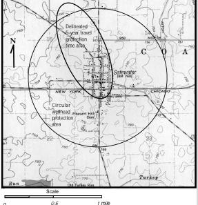
Figure 1. The shortcut, fixed radius, method of delineation may save time and money in the short term, but it is less accurate and often results in deliniating a larger wellhead protection area than a modeled delineation.
